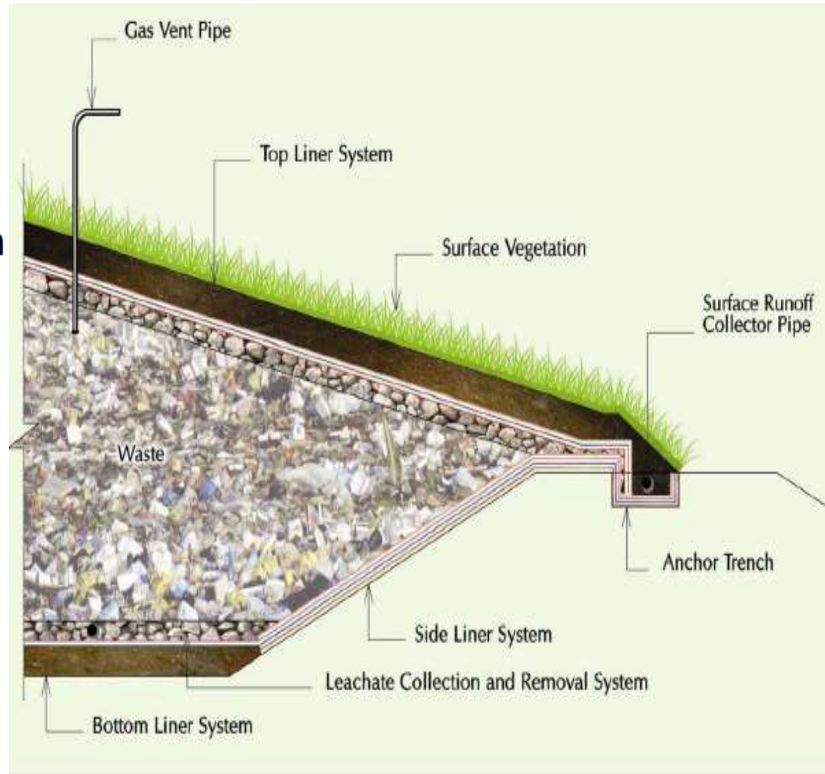
Typical Cross-Section of Landfill
