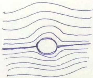
Potential flow streamline about a thin plate attached to a cylinder. (fig 1)
