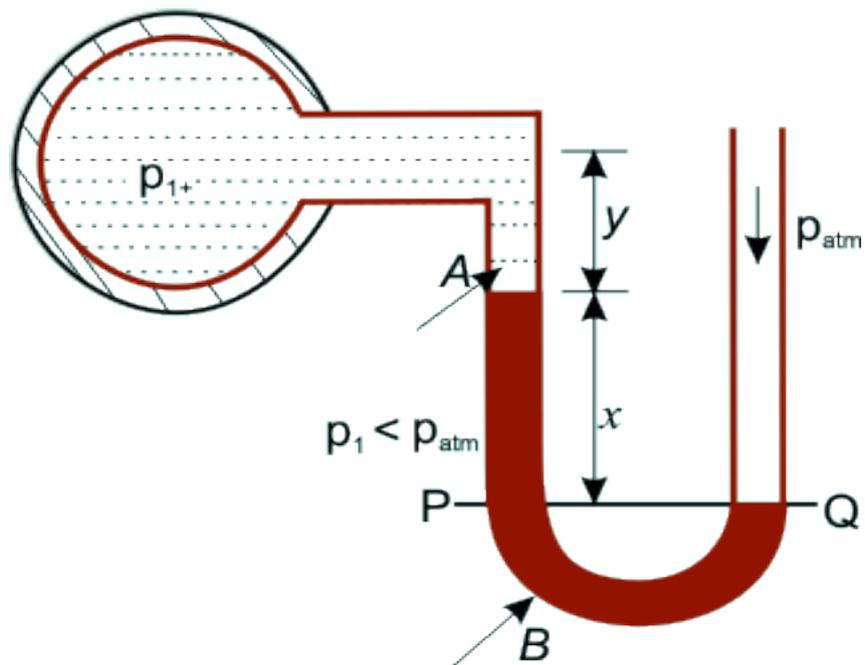
**Simple manometer to measure vacuum pressure****SINGLE COLUMN MANOMETER**
