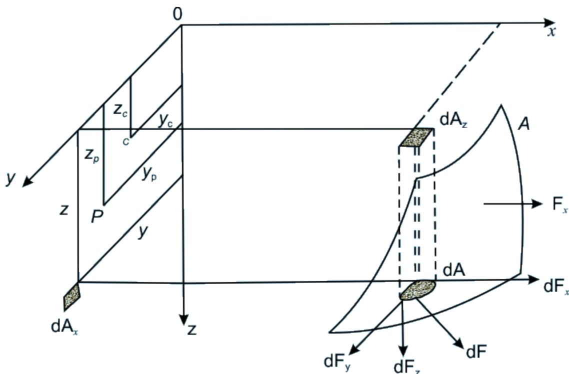
Consider an elemental area  $dA$  at a depth  $z$  from the surface of the liquid. The hydrostatic force on the elemental area  $dA$  is
