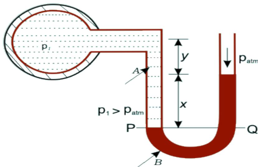
**Simple manometer to measure gauge pressure**
