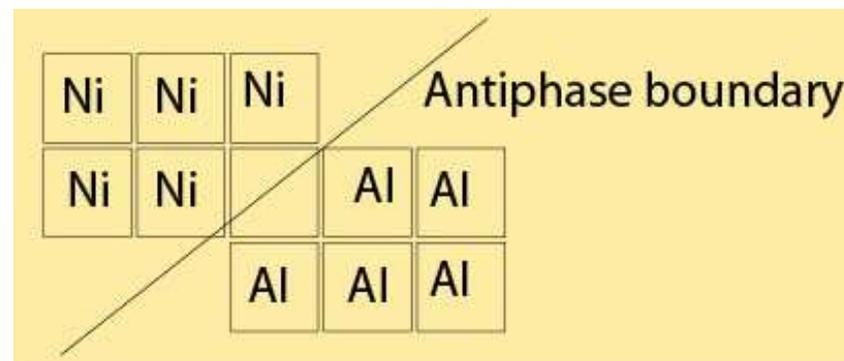
The schematic of the formation of antiphase boundaries in an ordered alloy due to the accidents of growth. <sup>375</sup>
