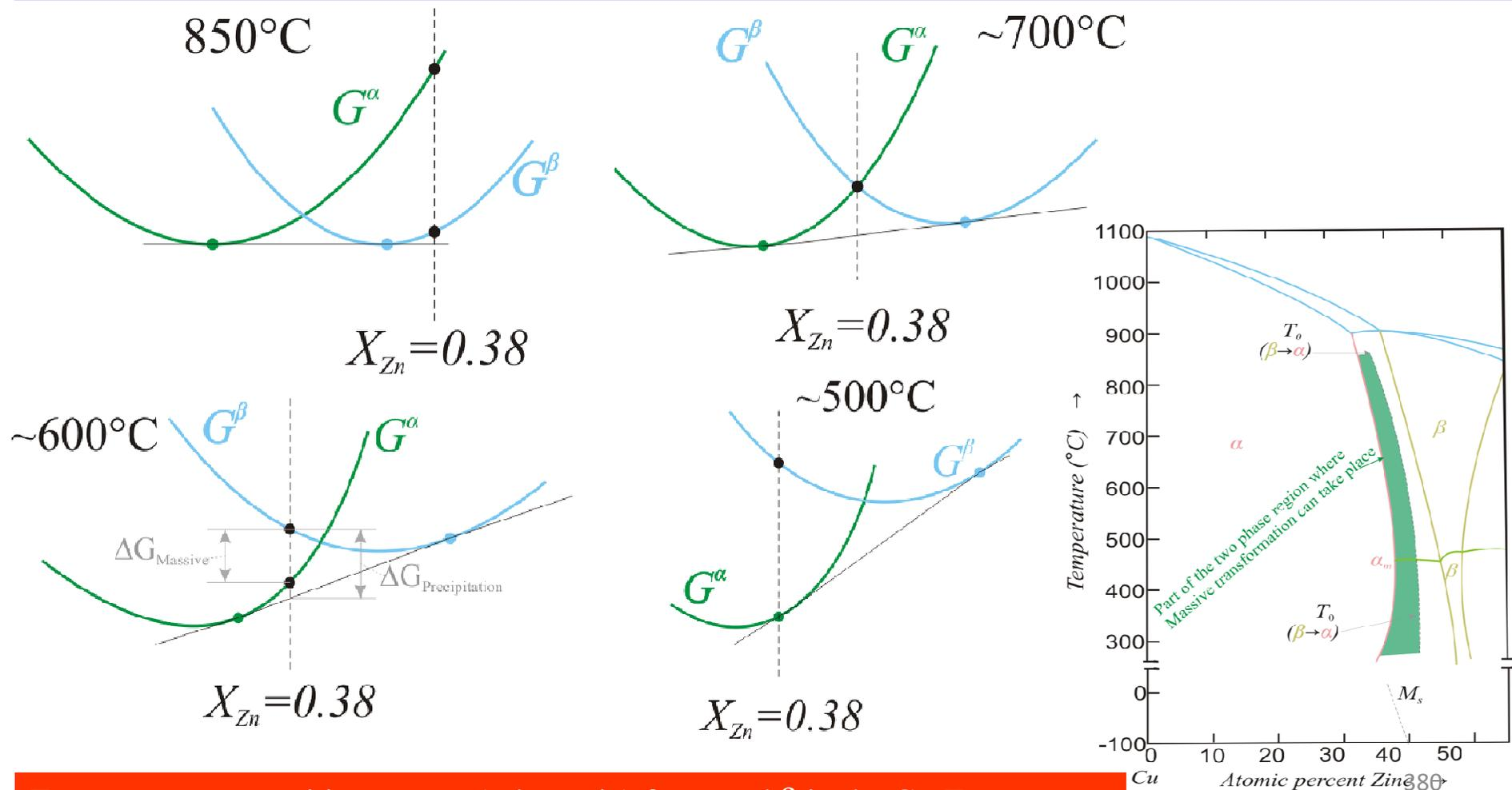
Free energy composition curves (schematic) for  $\alpha$  and  $\beta$  in the Cu-Zn system
