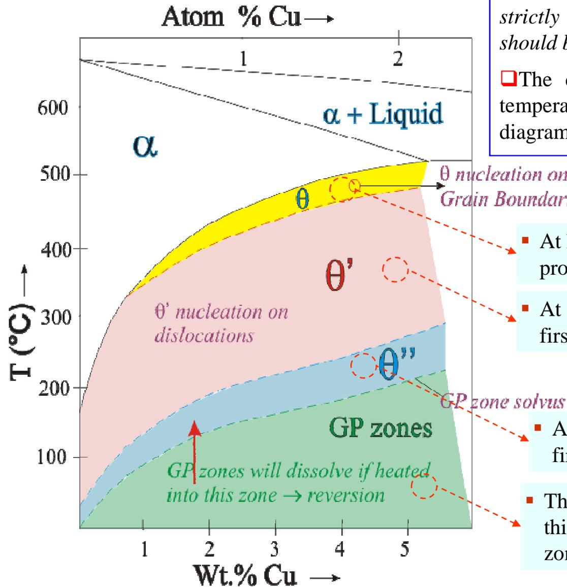
□ In this diagram additionally information has been superposed onto the phase diagram (*which strictly do not belong there- hence this diagram should be interpreted with care*)
