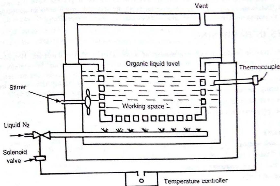
Figure : Liquid cooled (liquid  $\text{N}_2$ ) system. Components are immersed in a bath of alcohol, or trichloro ethylene, which is cooled by a submerged liquid nitrogen spray ( $-150^\circ\text{C}$ ), cooling rates can be controlled.
