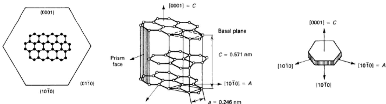
Crystalline structure of graphite, A and C possible growth directions
