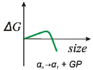
*If the transformation is broken down into a series of steps with smaller activation barrier the processes can take place even with low thermal activation*
