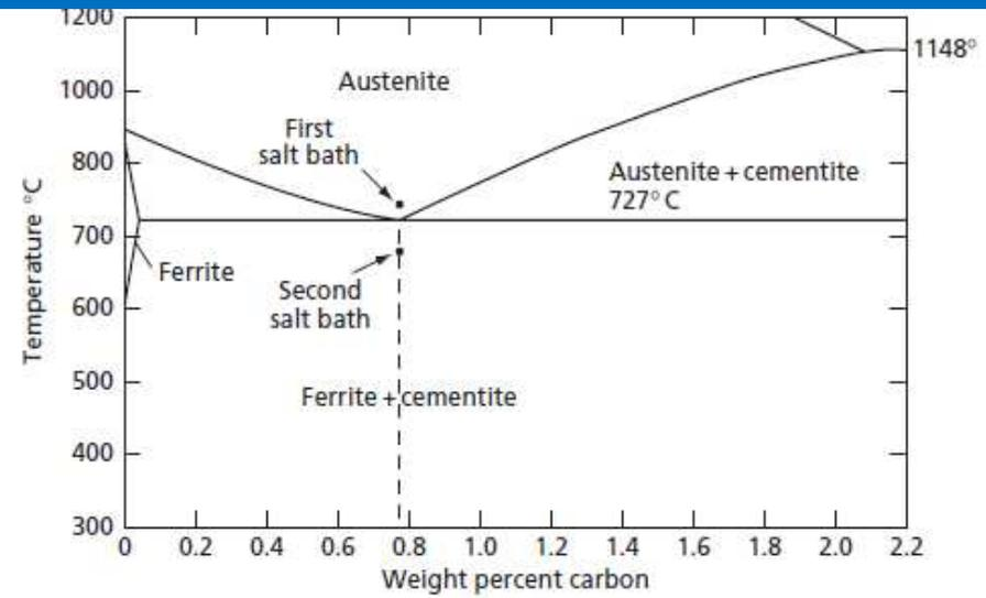
Eutectoid section of the iron - carbon diagram
