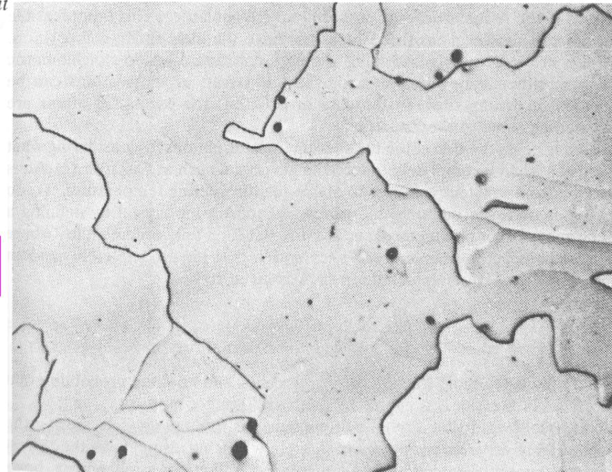
Massive  $\alpha$  in an Fe-0.002 wt% C quenched into iced brine from 1000  $^{\circ}$ C. Note the irregular  $\alpha/\alpha$  boundaries. (After T.B. Massalski in *Metals Handbook*, 8th edn., Vol. 8, American Society for Metals, 1973, p. 186.)
