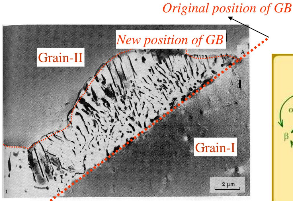
Cellular precipitation of  $Mg_{17}Al_{12}$  in an Mg-9 at% Al alloy solution treated and aged 1 h at 220 °C followed by 2 min at 310 °C. Some general  $Mg_{17}Al_{12}$  precipitation has also occurred on dislocations within the grains.
