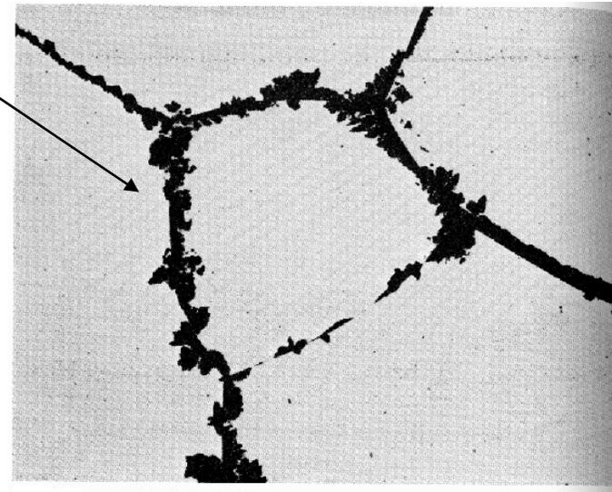
A partially transformed eutectoid steel. Pearlite has nucleated on grain boundaries and inclusions ( $\times 100$ ). (After J.W. Cahn and W.C. Hagel in *Decomposition of Austenite by Diffusional Processes*, V.F. Zackay and H.I. Aaronson (Eds.), 1962, by permission of The Metallurgical Society of AIME.)
