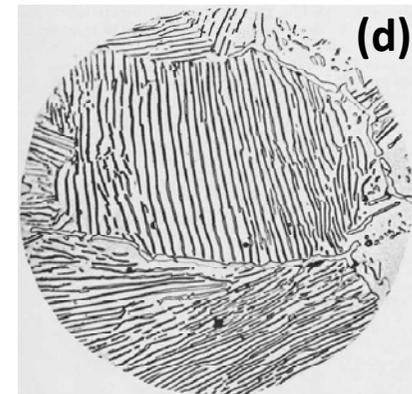
Fig. d: Hypereutectoid-steel microstructure. Notice the band of cementite plates outlining the pearlite colony in the center of the photograph. 1000X
