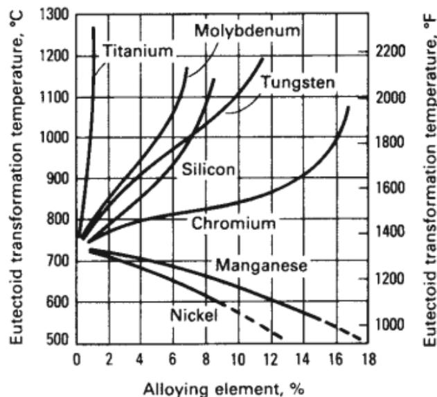
Effect of alloying element on eutectoid temperature
