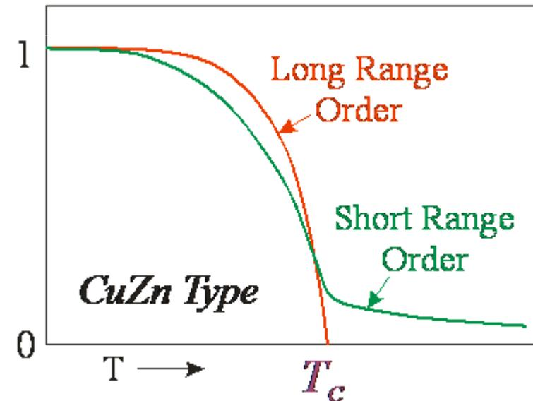
Order parameter variation with temperature: continuous ( $B_2$  type) and abrupt ( $L1_2$ ).
