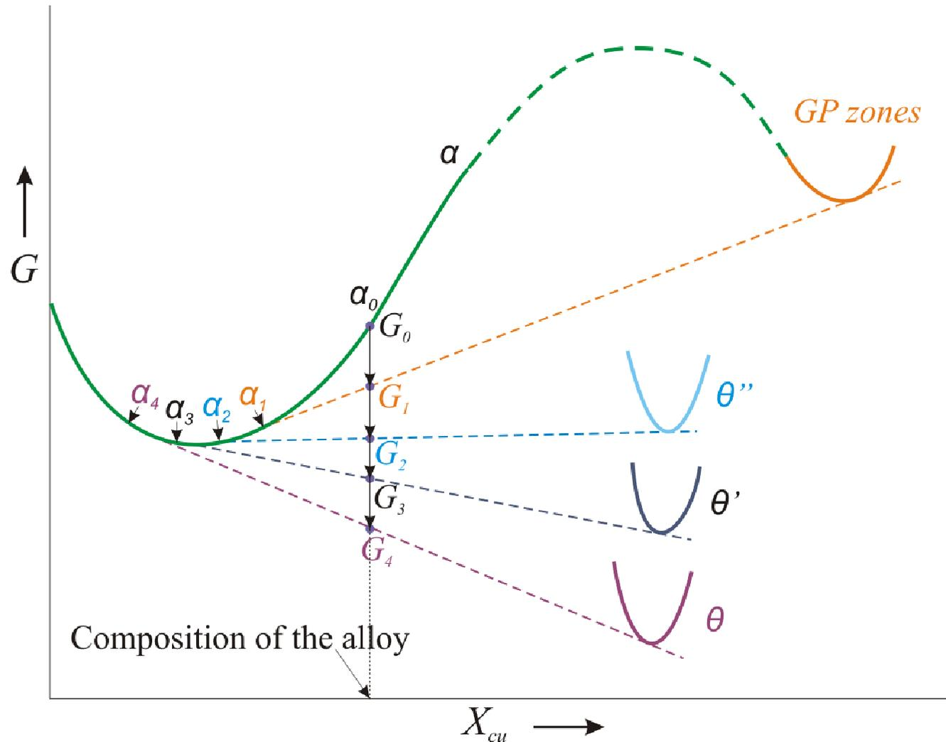
Schematic diagram showing the lowering of the Gibbs free energy of the system on sequential transformation:
