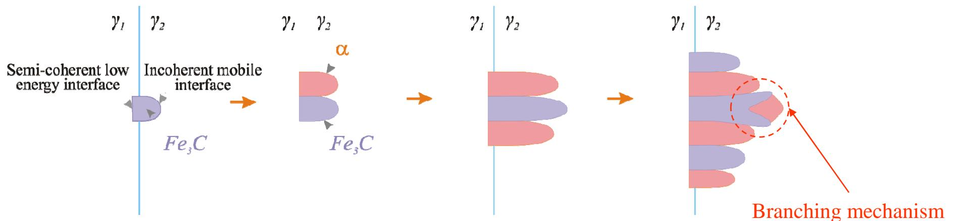
Nucleation of the eutectoid phases in a system with eutectoid composition
