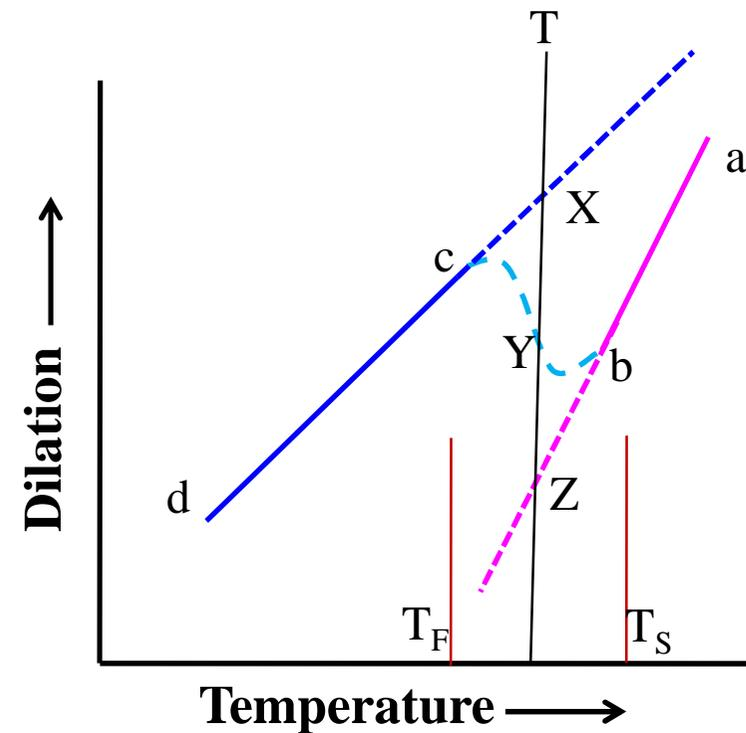
Fig. b : Dilation-temperature plot for a cooling curve
