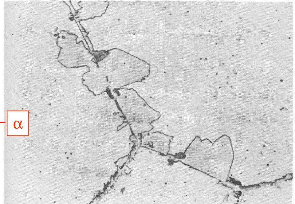
Massive  $\alpha$  formed at the grain boundaries of  $\beta$  in Cu-38.7 wt% Zn quenched from 850  $^{\circ}\text{C}$  in brine at 0  $^{\circ}\text{C}$ . Some high temperature precipitation has also occurred on the boundaries. (From D. Hull and K. Garwood, *The Mechanism of Phase Transformations in Metals*, Institute of Metals, London, 1956.)
