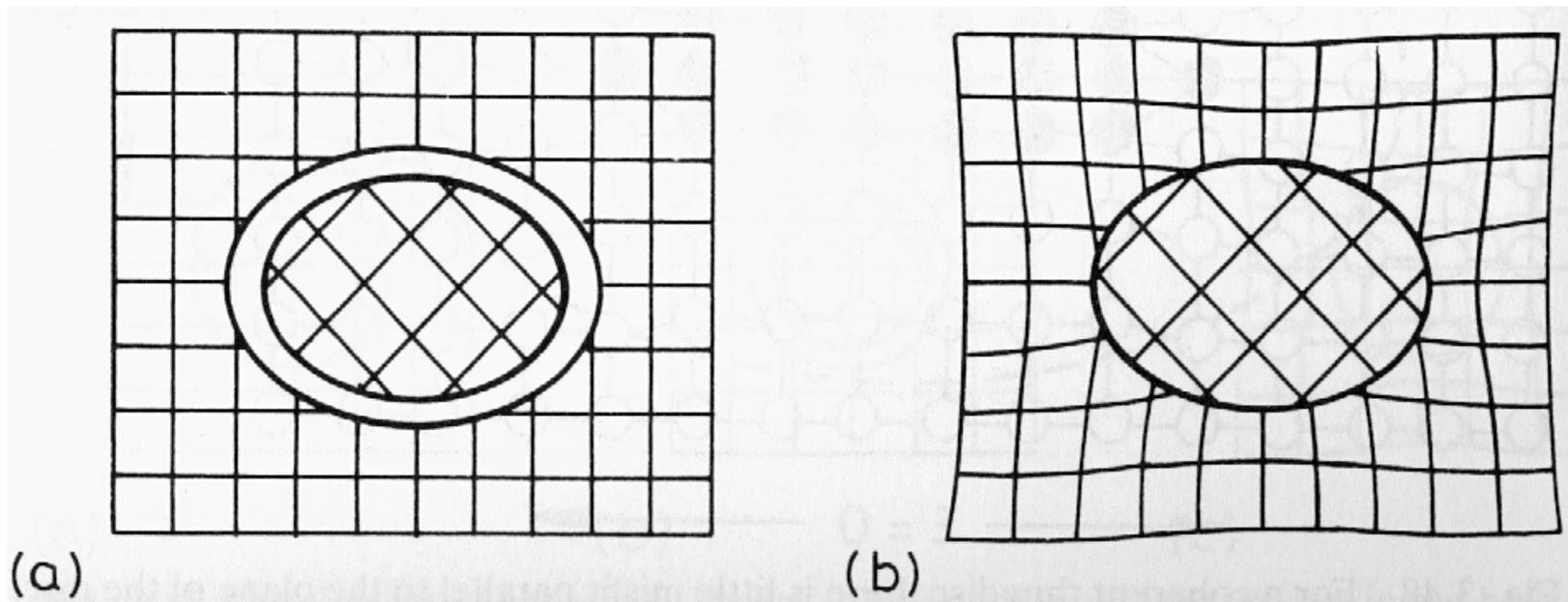
The origin of misfit strain for an incoherent precipitate (no lattice matching) <sup>327</sup>
