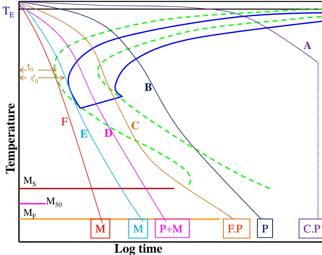
$t_0$  = Minimum incubation period at the nose of the TTT diagram,
