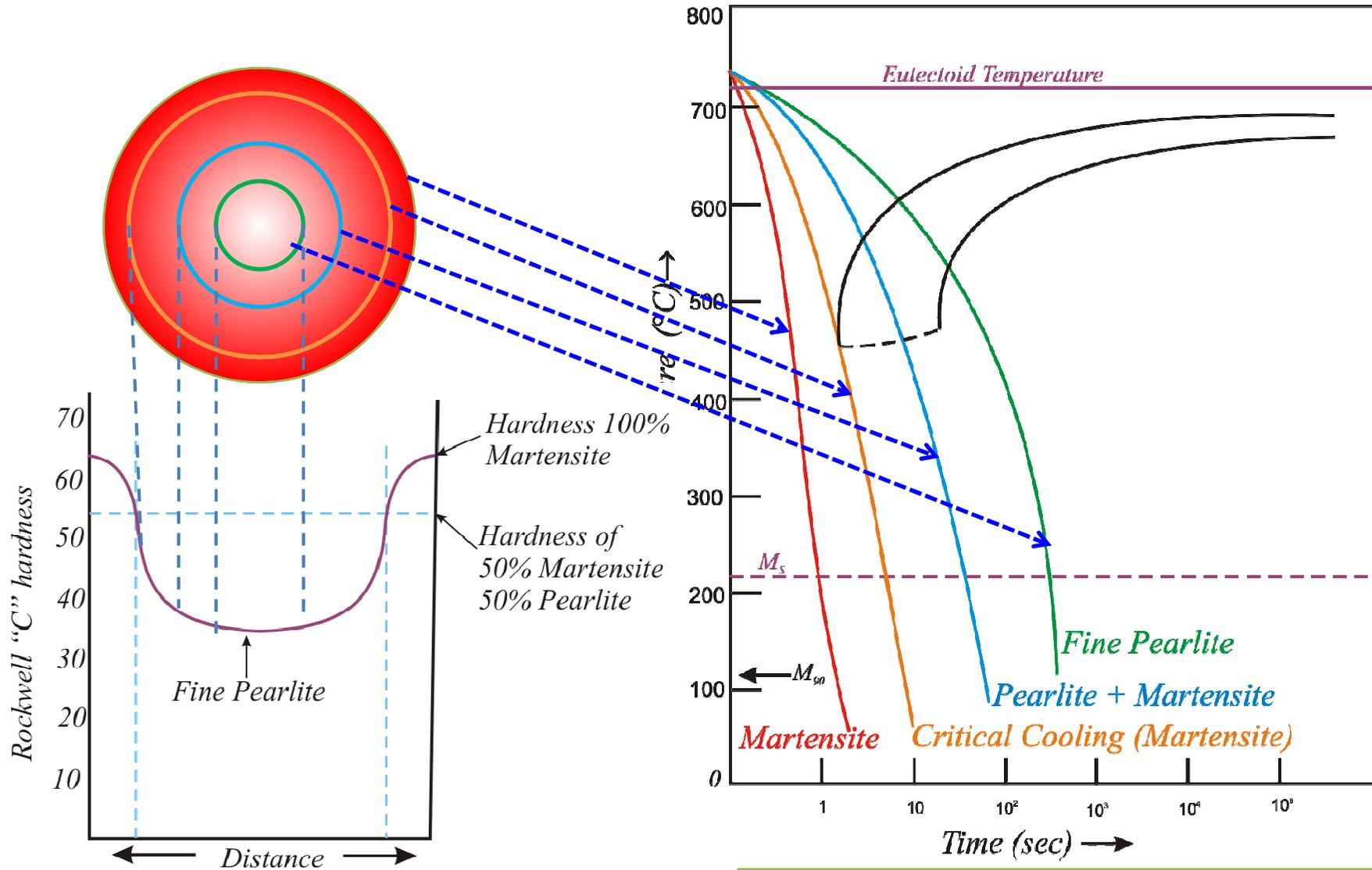
Typical hardness test survey made along a diameter of a quenched cylinder
