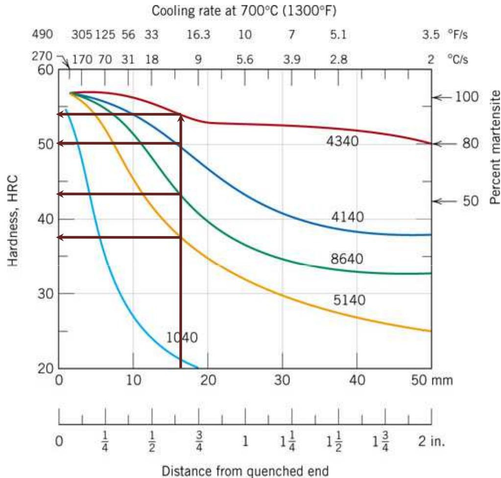
Hardness at center of a 3 inch bar is different for different steels indicating different amounts of martensite at the center
