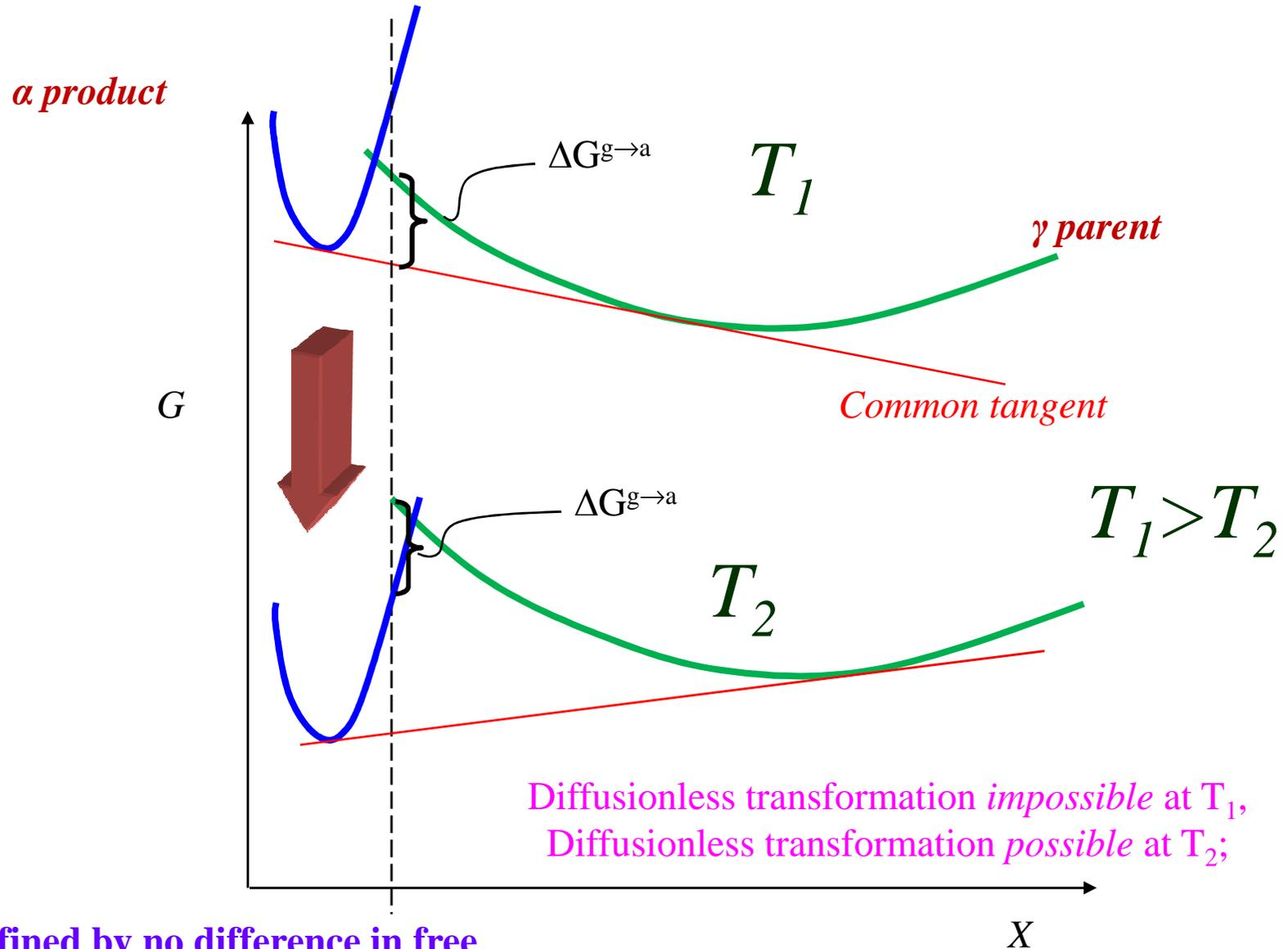
“ $T_0$ ” is defined by no difference in free energy between the phases,  $\Delta G=0$ .
