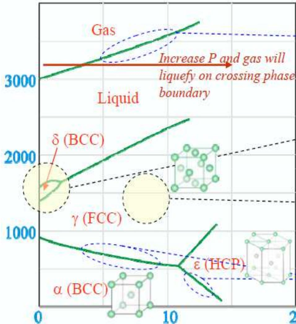
This line slopes upward as at constant T if we increase the P the gas will liquefy as liquid has lower volume (similarly the reader should draw horizontal lines to understand the effect of pressure on the stability of various phases- and rationalize the same).
