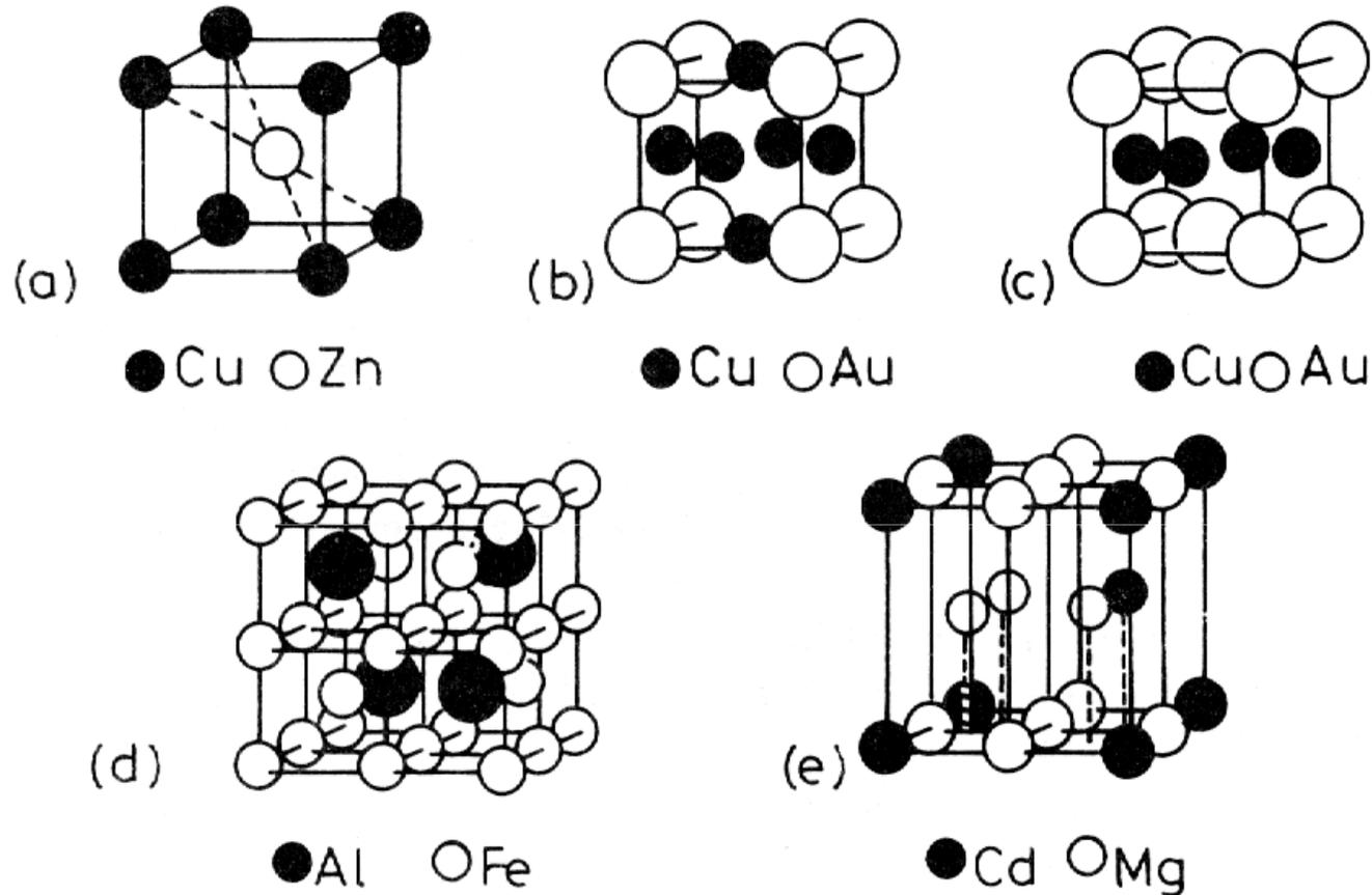
The five common ordered lattices, examples of which are: (a)  $L2_0$ : CuZn, FeCo, NiAl, FeAl, AgMg; (b)  $L1_2$ :  $Cu_3Au$ ,  $Au_3Cu$ ,  $Ni_3Mn$ ,  $Ni_3Fe$ ,  $Ni_3Al$ ,  $Pt_3Fe$ ; (c)  $L1_0$ : CuAu, CoPt, FePt; (d)  $D0_3$ :  $Fe_3Al$ ,  $Fe_3Si$ ,  $Fe_3Be$ ,  $Cu_3Al$ ; (e)  $D0_{19}$ :  $Mg_3Cd$ ,  $Cd_3Mg$ ,  $Ti_3Al$ ,  $Ni_3Sn$ . (After R.E. Smallman, *Modern Physical Metallurgy*, 3rd edition, Butterworths, London, 1970.)
