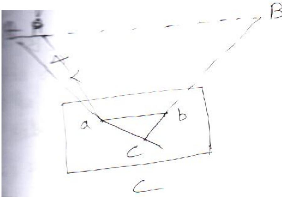
1. Let 'C' be the instrument station to be located on the plan. Let 'A' and 'B' be two visible stations which have been plotted on the sheet as 'a' and 'b'. set the table at 'c' and orient it with compass. Clamp the table.
