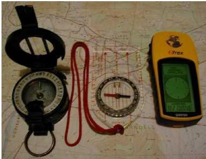
Compass surveys are mainly used for the rapid filling of the detail in larger surveys and for explanatory works. It does not provide a very accurate determination of the bearing of a line as the compass needle aligns itself to the earth's magnetic field which does not provide a constant reference point.
