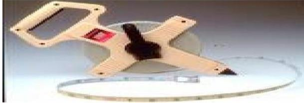
**i. Linen or Linen with steel wire woven into the fabric;**
