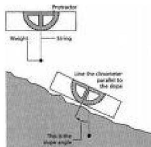
This instrument is used for measuring angles of ground slopes (slope angle). They are of several form, the common form is the **WATKING'S CLINOMETER**, which consist of a small disc of about 60mm diameter. A weighted ring inside the disc can be made to hang free and by sighting across this graduated ring angle of slopes can be read off. It is less accurate than abney level.
