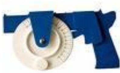
This instrument is generally used to obtaine roughly the slope angle of the ground. It consists of a rectangular, telescopic tube (without lenses) about 125mm long with a graduated arc attached. A small bubble is fixed to the vernier arm, once the image of the bubble is seen reflected in the eyepiece the angle of the line of sight can be read off with the aid of the reading glass.
