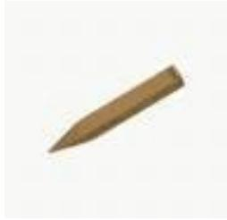
Pegs are made of wood 50mm x 50mm and some convenient length. They are used for points which are required to be permanently marked, such as intersection points of survey lines. Pegs are driven with a mallet and nails are set in the tops.
