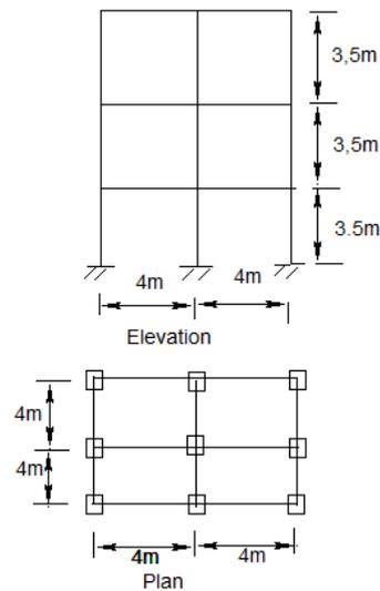
Figure 10.2.1 Plan and elevation of multi-storey building
