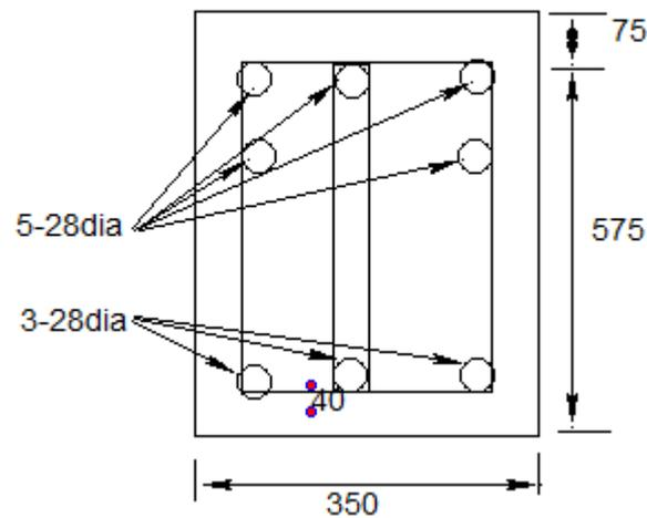
Figure 8.2.1 Details of doubly reinforced beam
