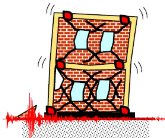
Figure 2.3 (c) Severe (Infrequent) Shaking – Structural damage, but NO collapse
