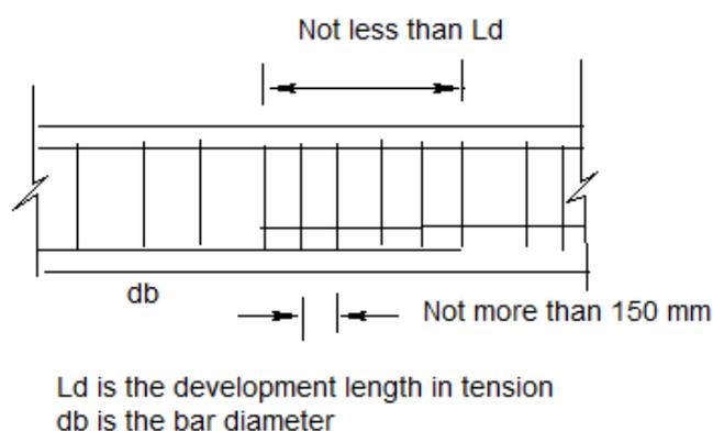
Figure 7.2 Lap, splice in beam
