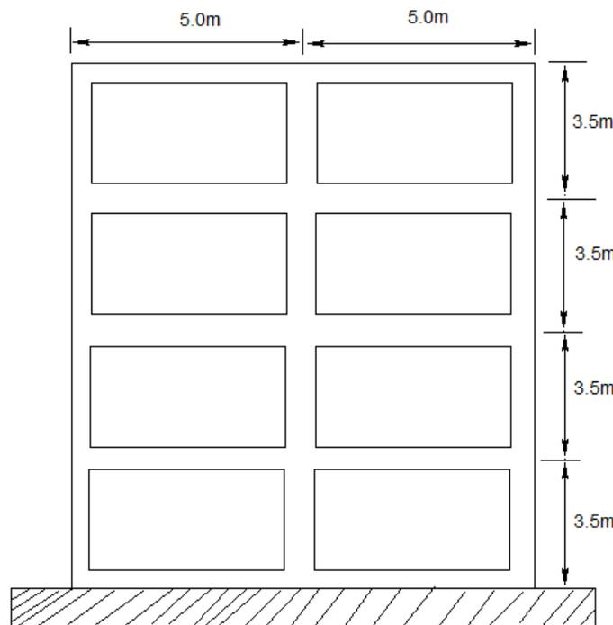
Figure 10.1.1 a: Plane frame structure (Four storeyed building)
