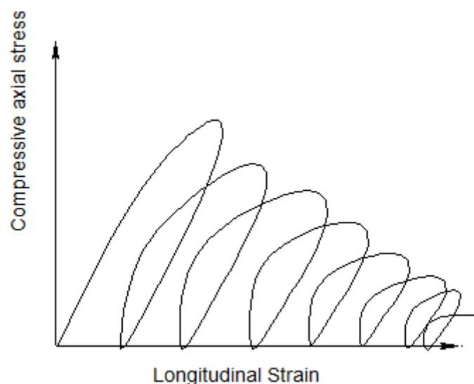
Figure 3.1 Plain concrete section under repeated compressive loading
