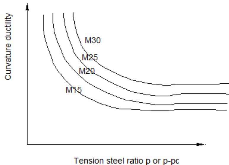
Figure 5.2 Curvature ductility in beams with Fe 415 steel
