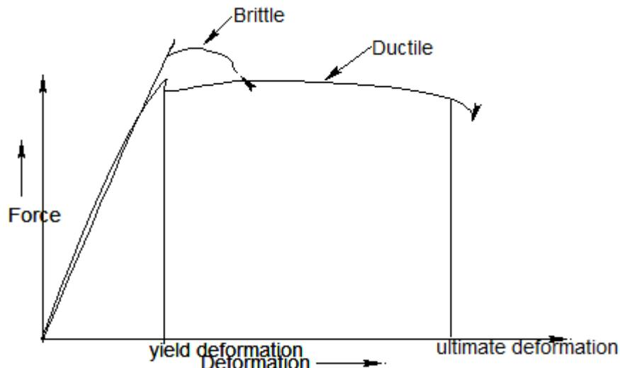
Figure 4.1 Brittle and ductile force deformation behaviour
