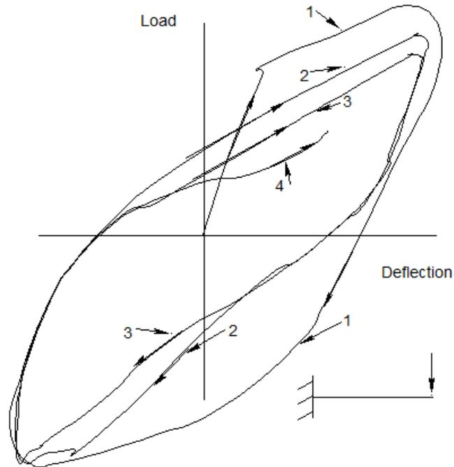
Figure 3.3 Hysteresis behaviour of a cantilever beam
