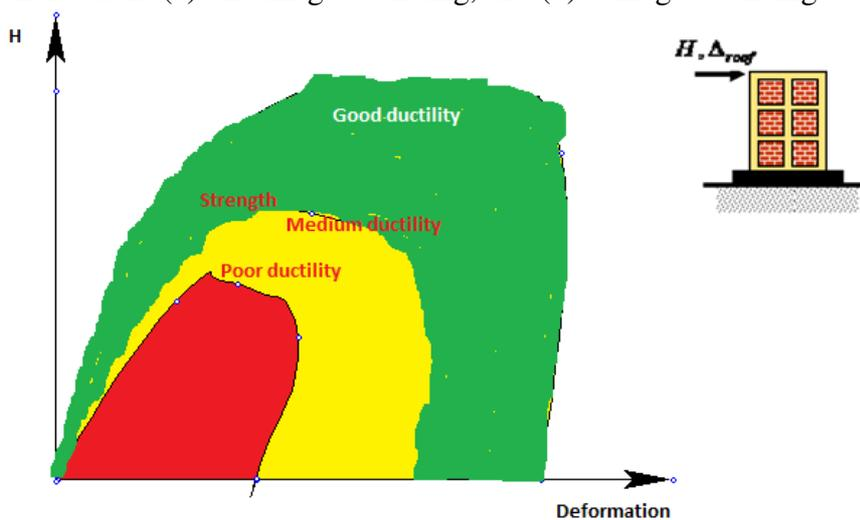
Figure 2.6 Ductility: Buildings are designed and detailed to develop favourable failure mechanisms that possess specified lateral strength, reasonable stiffness and, above all, good post-yield deformability.
