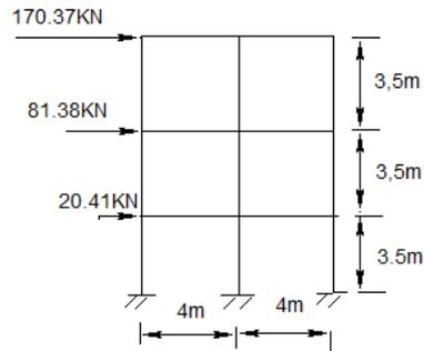
Figure 10.2.2 Design seismic forces by static analysis
