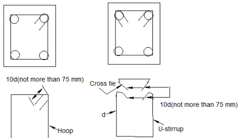
Figure 7.3 Beam web reinforcement
