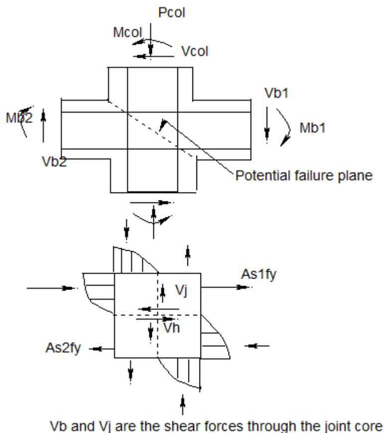
Figure 6.2 Forces on an interior beam-column joint
