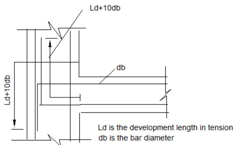
Figure 7.1 Anchorage of beam bars in an external joint
