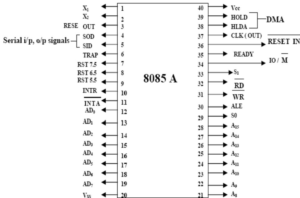
Fig. 6 8085 microprocessor pin layout and signal groups
