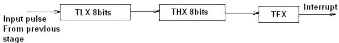
Fig 4.19 Operation of Timer in Mode 1
