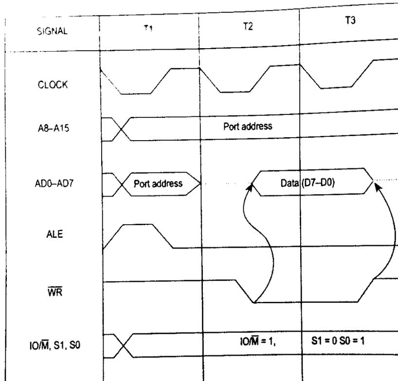
Fig. 11 Timing diagram I/O write machine cycle
