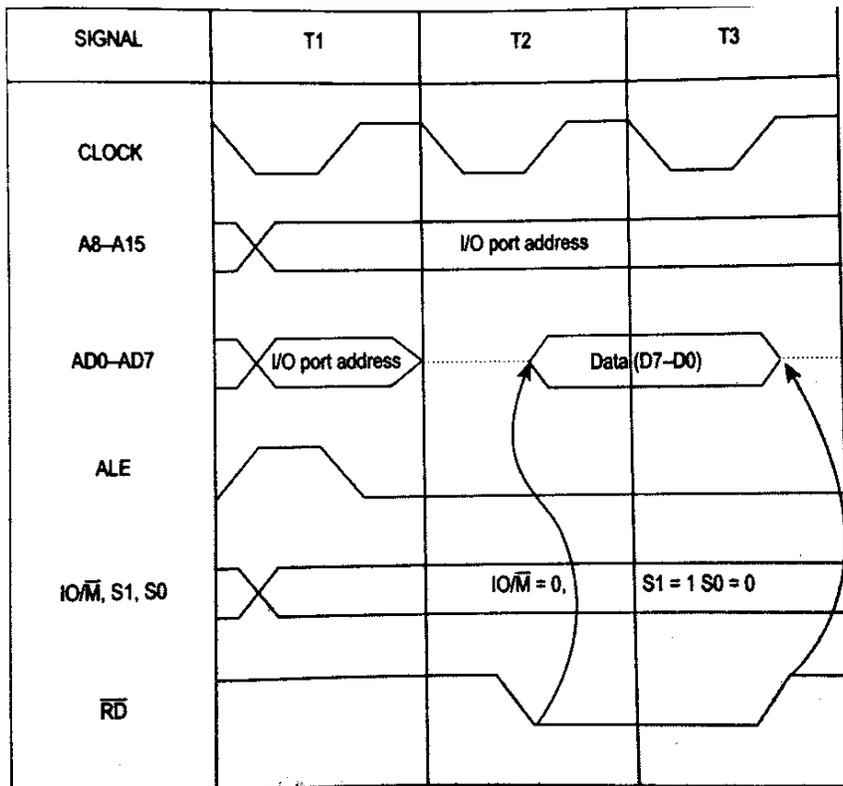
Fig. 10 Timing diagram I/O read machine cycle
