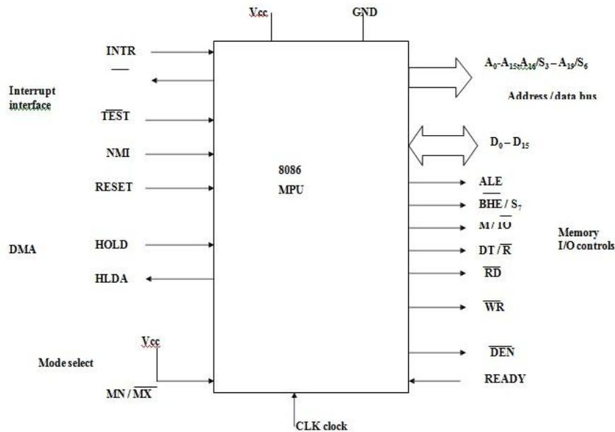
Block Diagram of the Minimum Mode 8086 MPU
