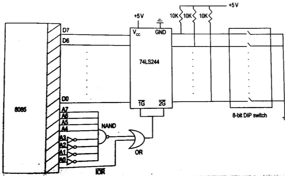
Fig. 21 interfacing of 8-bit DIP switch with 8085
