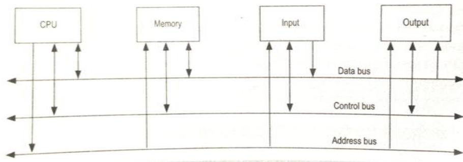
Fig.1 Microprocessor-based system
