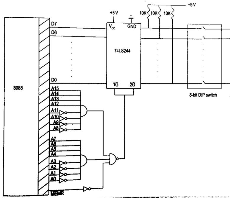
Fig. 22 Interfacing 8-bit DIP switch with 8085
