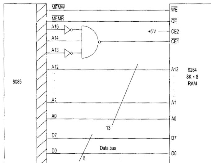
Fig. 18 Interfacing 6264 IC with the 8085
