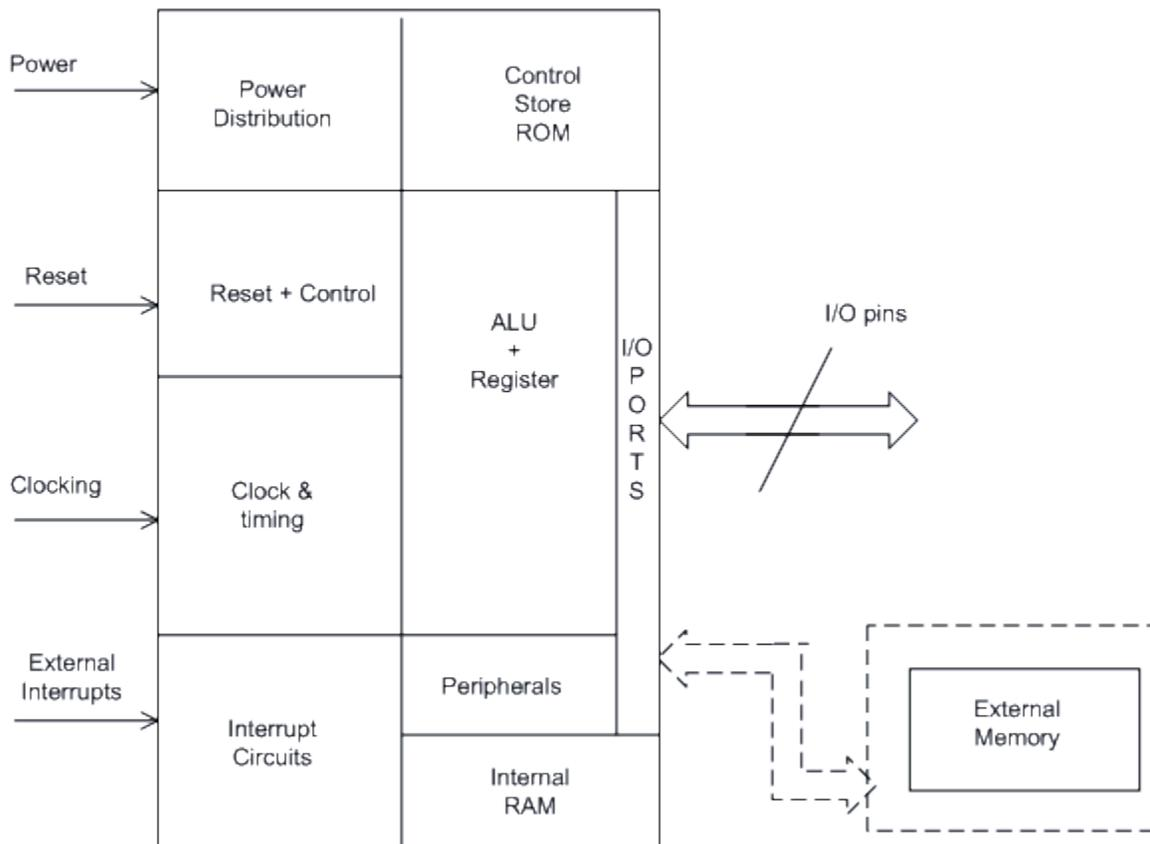
Fig. 4.1 Internal Structure of a Microcontroller
