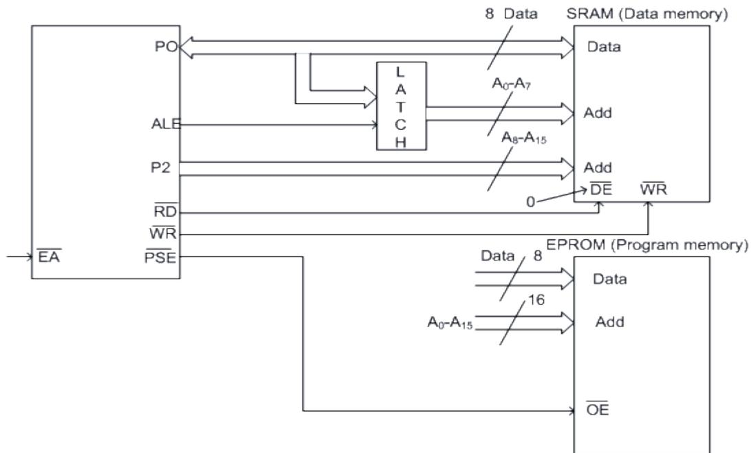
Fig 4.9: Circuit Diagram for Interfacing of External Memory
