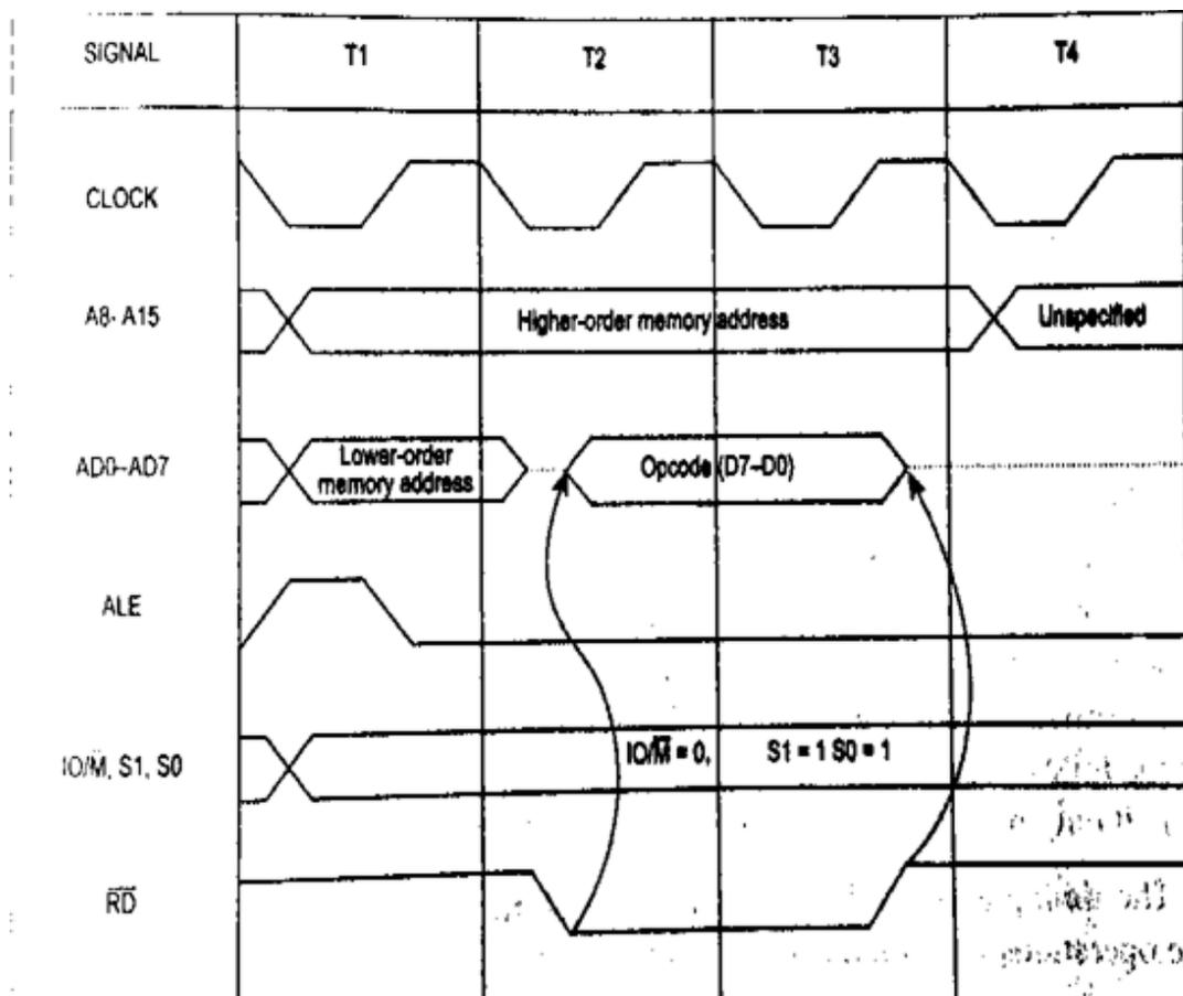
Fig. 7 Timing diagram for opcode fetch cycle
