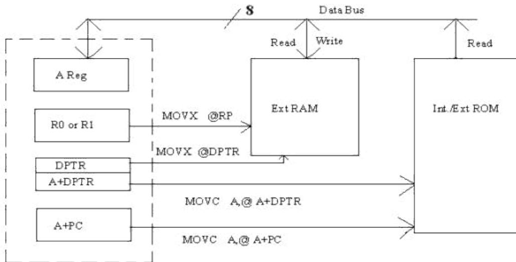
Fig 4.14 Schematic diagram of external memory access
