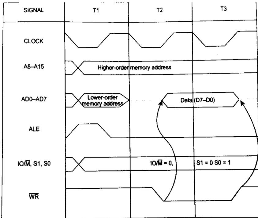
Fig. 9 Timing diagram for memory write machine cycle
