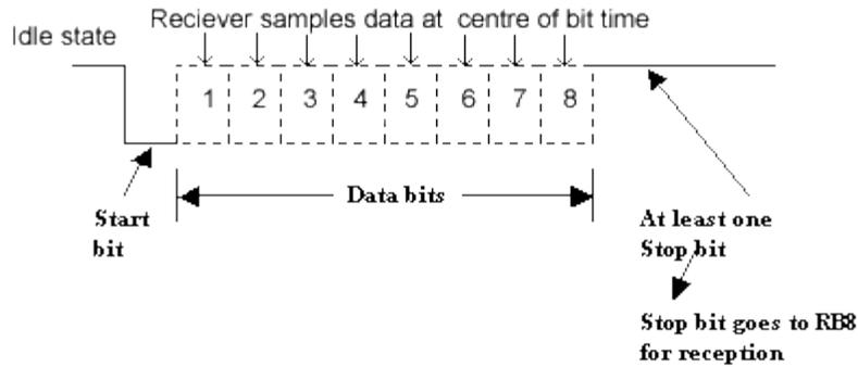
Fig 4.26 Data transmission format in UART mode
