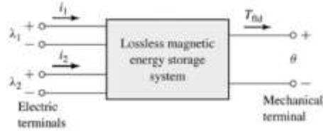
**Fig. 1.7 Multiply-excited magnetic energy storage system**
