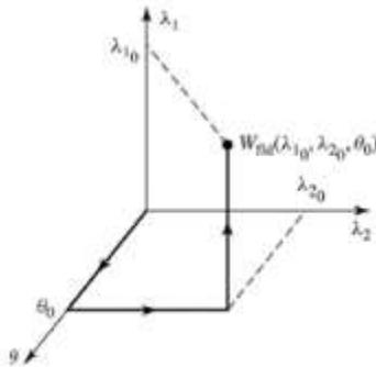
**Fig. 1.8 Integration path to obtain  $W_{\text{fld}}(\lambda_{1_0}, \lambda_{2_0}, \theta_0)$**
