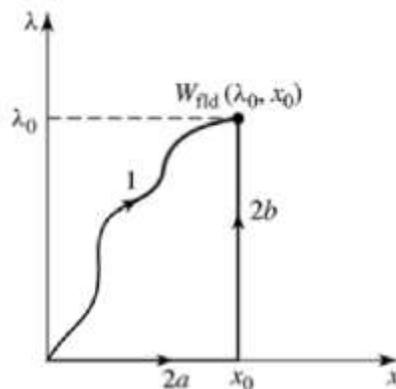
Fig. 1.5 Integration paths for  $W_{\text{fld}}$
