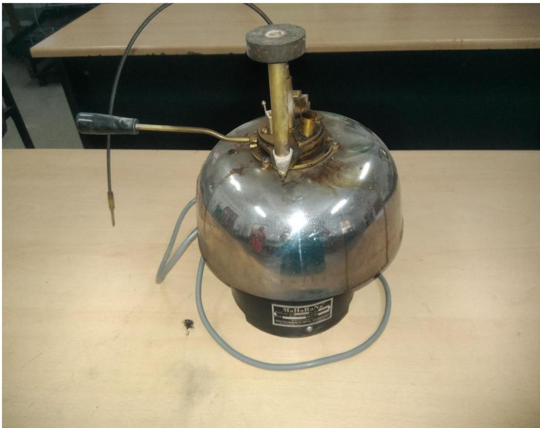
**FLASH POINT AND FIRE POINT APPARATUS**
