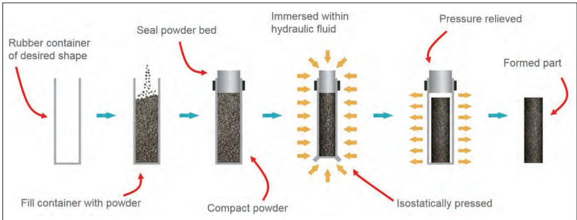
*Fig.1. Schematic of a Cold Isostatic Pressing (CIP) process*
