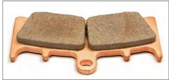
*Figure 6: Motorcycle brake lining. Copper-plated carrier (bottom) and two sintered friction linings. The two materials are bonded during sintering without the use of auxiliary materials, and the sintering of the friction lining does not require any subsequent calibration.*
