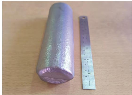
Fig. 3: Oval cross section indicating excessive slumping
