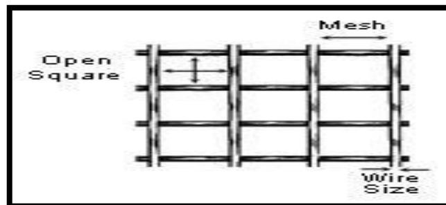
Fig. 3: Illustration of square openings
