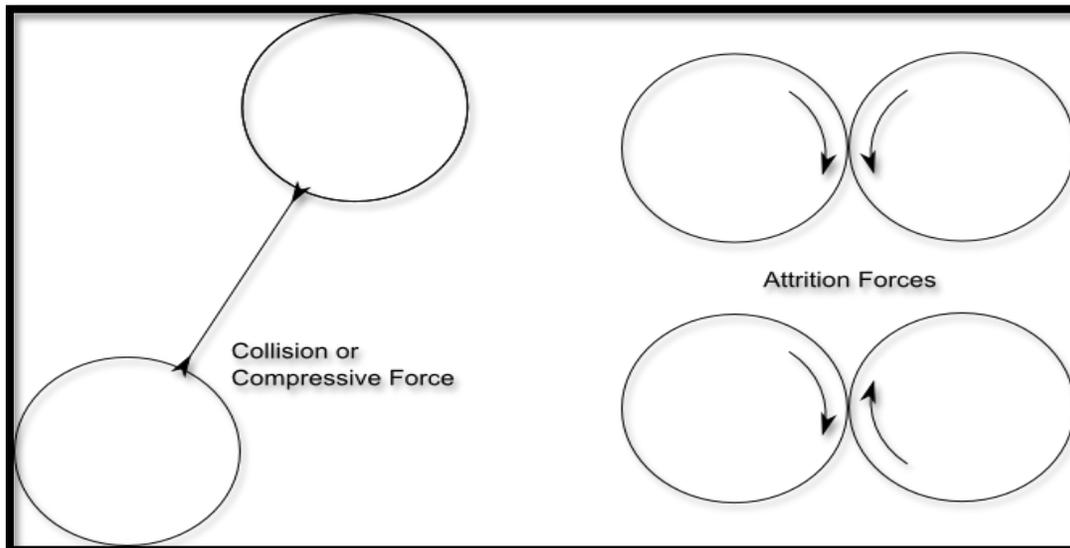
**Fig. 10: Schematic Diagram of Different Type of forces during Ball Mill Operation**
