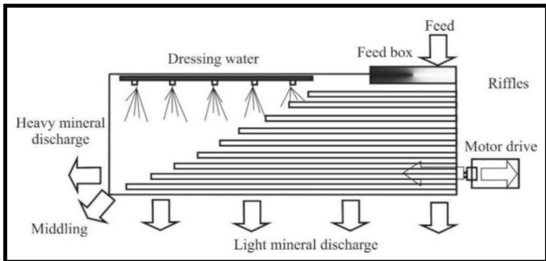
**Fig 12: Schematic Diagram of Wilfley Table**
