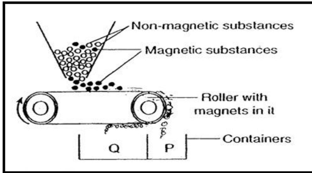
Fig 15: Schematic Diagram of Magnetic Separation
