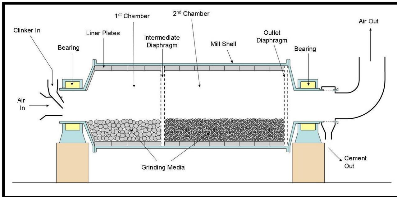
Fig. 8: Schematic Diagram of a Cylindrical Ball Mill
