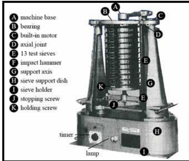
**Fig. 4: Illustration of a Ro-Tap Sieve Shaker**
