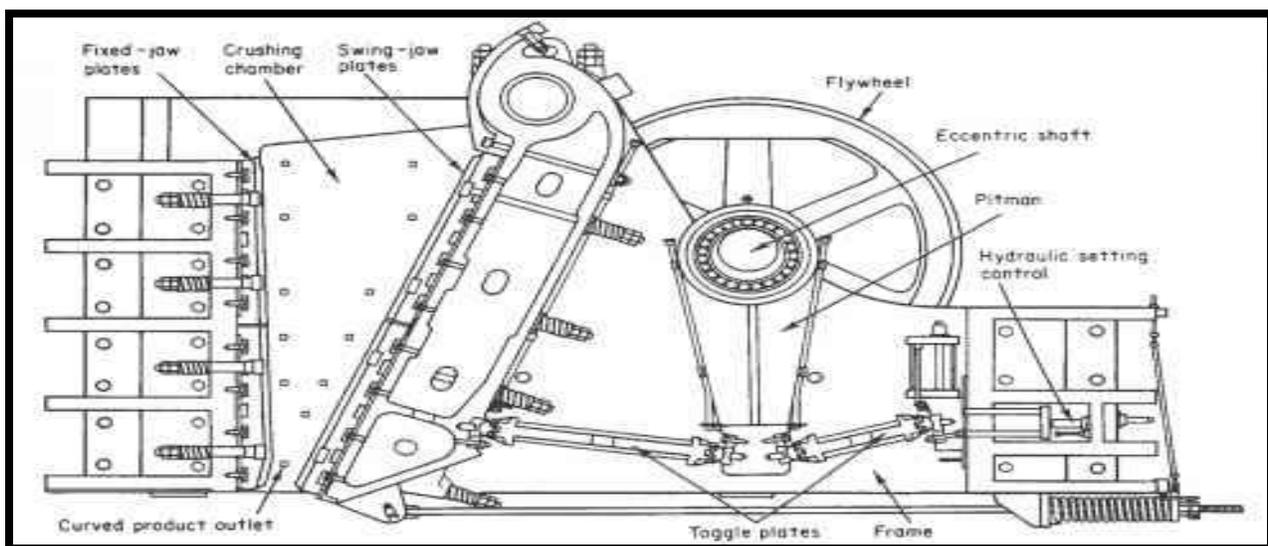
Fig. 5: Schematic diagram of Blake Jaw Crusher
