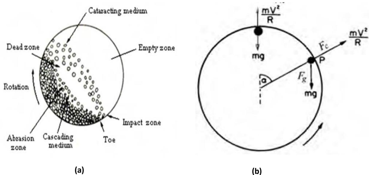
Fig. 11: (a) Different Stages & zones of a Ball mill (b) Forces working on the Grinding media
