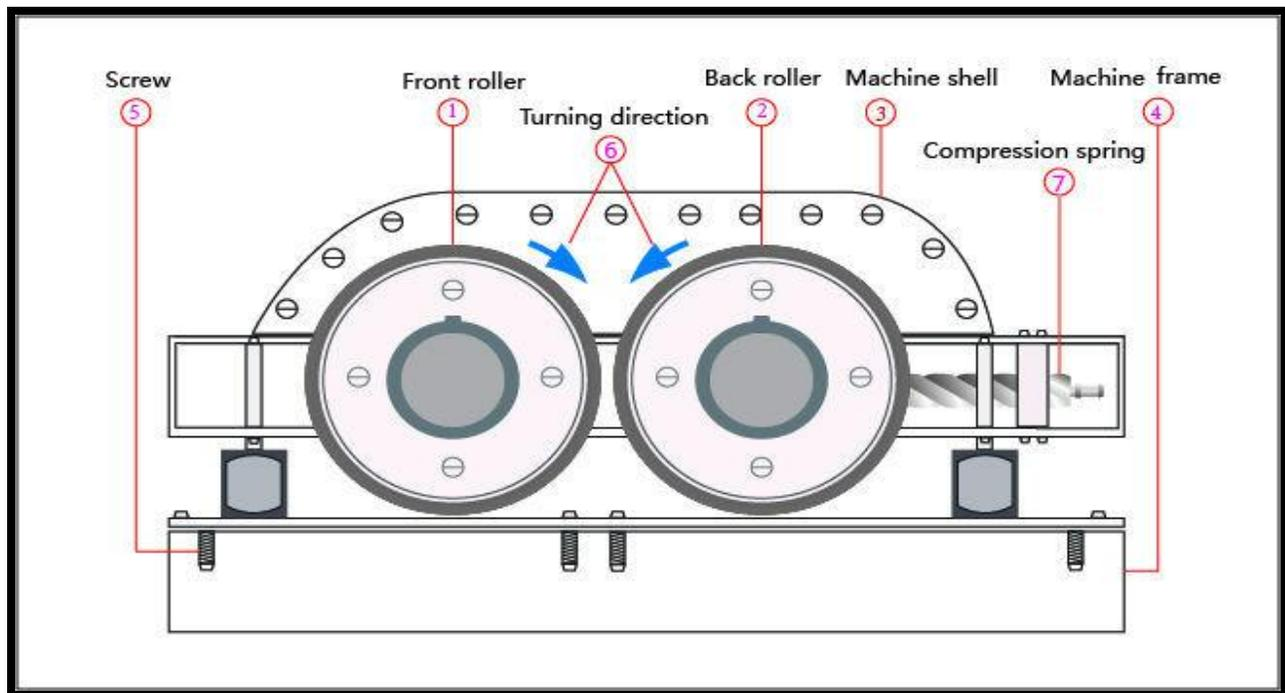
**Fig. 7: Schematic Diagram of Roll Crusher**
