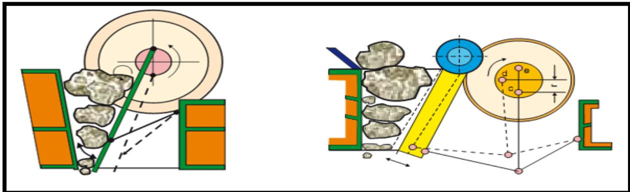
Fig. 6: Schematic Diagram of Crushing Operation in Blake Jaw Crusher
