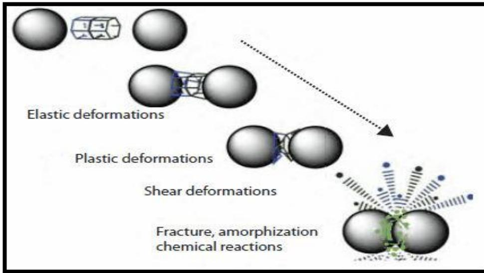
**Fig. 9: Schematic Diagram of Different forms of Deformation during Ball-powder Interaction**
