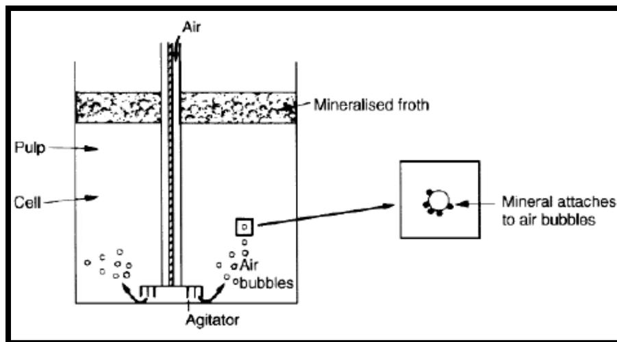
**Fig. 13: Schematic Diagram Flotation Process**
