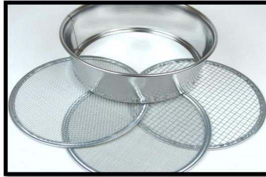
**Fig.2: Test Sieves of different sizes**
