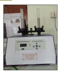
**1.Tap Density Apparatus:** settling/tapping apparatus, graduated cylinders
