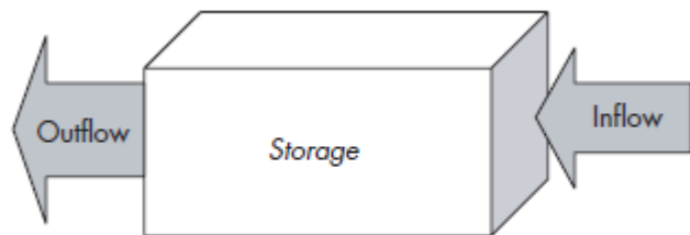
Figure 4.1 Illustration of the storage term used in the water balance equation.
