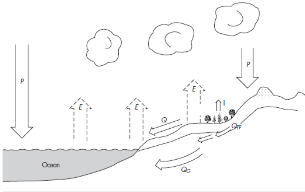
Figure 1.9 Processes in the hydrological cycle operating at the basin or catchment scale. Q = runoff; the subscript G stands for groundwater flow; TF for throughflow; I = interception; E = evaporation; P = precipitation.
