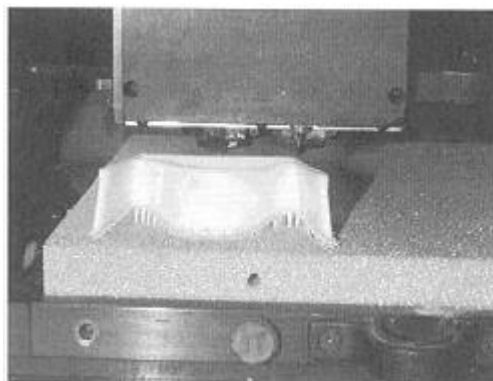
Figure 2.12 After 1 hour the model has built over 1-inch tall. Notice the part is being built hollow in order to speed up the process.
