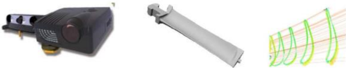
Figure 7: Optical 3D digitizer Nub3D Triple (Spain) (left); measured turbine blade (center); profile analysis (right).
