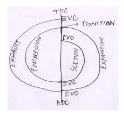
Fig. 4. Theoretical valve timing diagram
