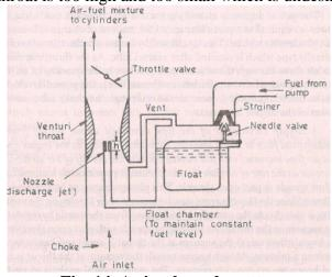
Fig. 14. A simple carburettor
