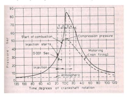
Fig. 27. Stages of combustion in CI engine
