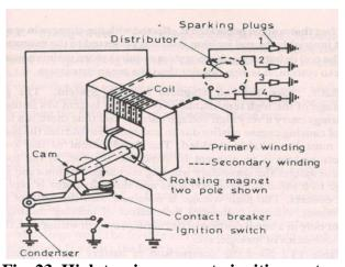
Fig. 23. High tension magneto ignition system
