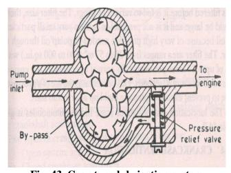
Fig. 43. Gear type lubrication system
