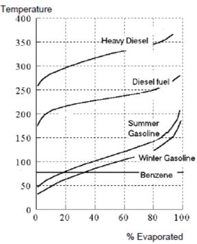
Fig. 12. Distillation curve
