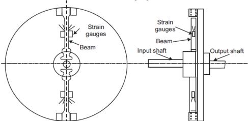
Fig. 33. Transmission dynamometer
