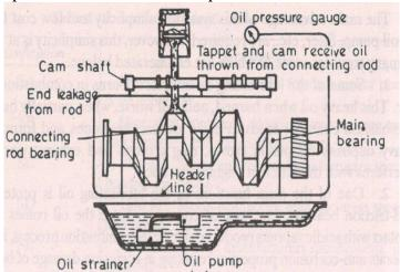
Fig. 42. Pressure lubricating system
