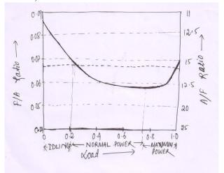
Fig. 13. Main areas of automotive engine operation
