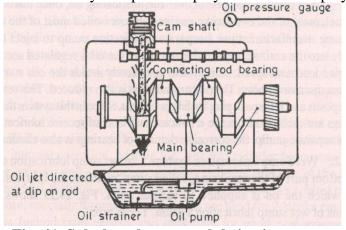
Fig. 41. Splash and pressure lubricating system
