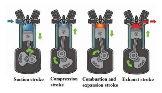
Fig. 2. Cycle of operation in four stroke engine
