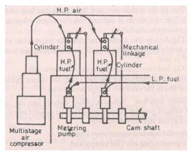
Fig. 17. Air injection system
