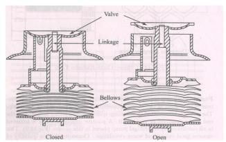
Fig. 38. Bellow type thermostat
