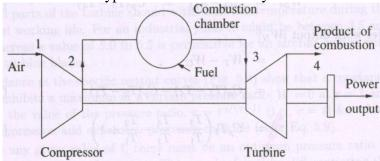
Fig. 44. Simple gas turbine
