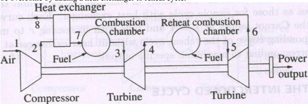
Fig. 47. Arrangement of reheat cycle with heat exchanger
