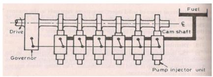
Fig. 19. Unit injector
