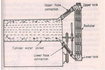
Fig. 37. Thermo-syphon cooling
