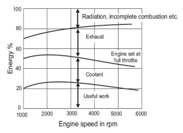
Fig. 35. Heat balance sheet for SI engine
