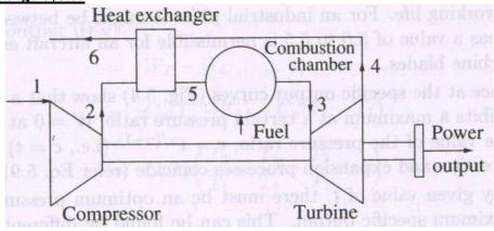
Fig. 45. Simple gas turbine with heat exchanger
