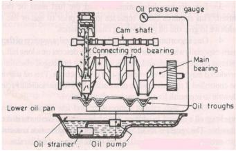
Fig. 40. Splash lubricating system
