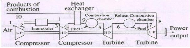
Fig. 49. Arrangement of intercooled cycle with heat exchanger and reheat
