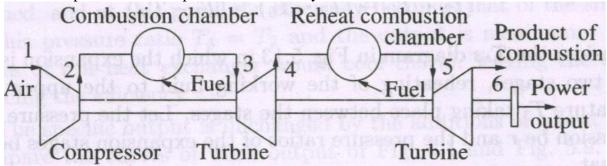
Fig. 46. Arrangement of reheat cycle
