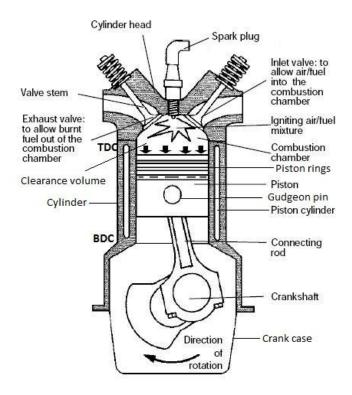
Fig. 1. Different parts of IC engine
