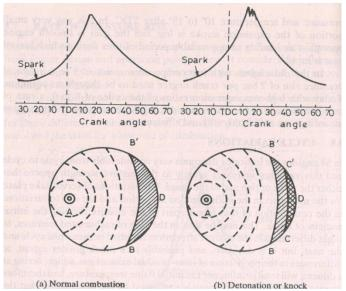
Fig. 26. Detonation in SI engine
