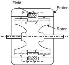
Fig. 32. Eddy current dynamometer
