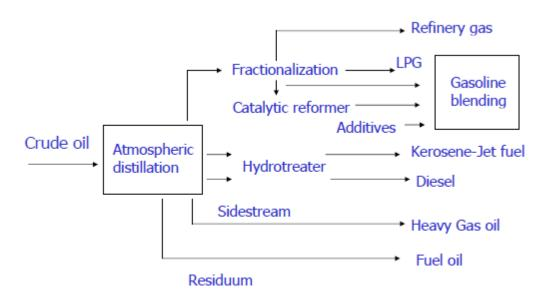
Fig. 10. Refinery processes
