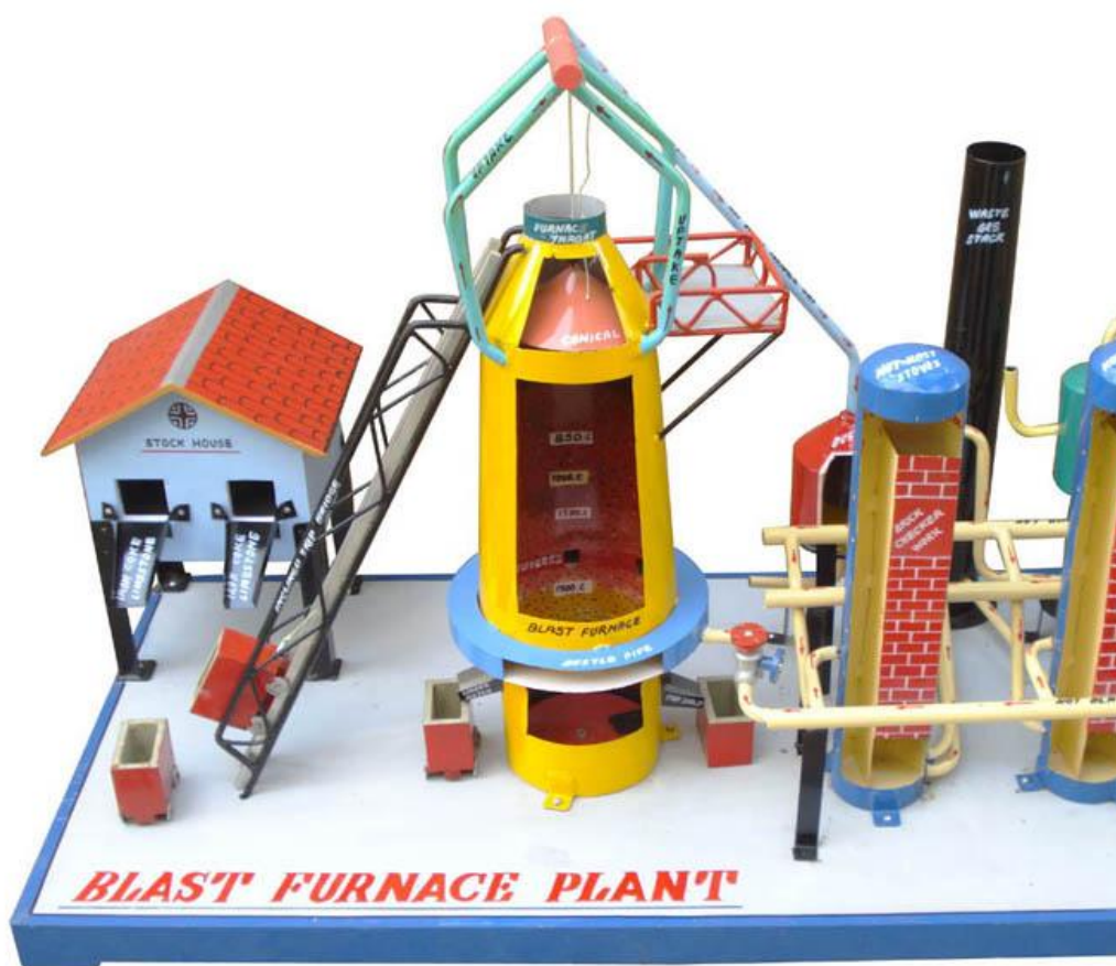
Figure 2.8 shows a schematic two-dimensional vertical section as illustration. Solid raw materials are stored in bins. Weighed quantities are loaded into the skip car, which goes up through inclined rail to the furnace top to off-load the charges.
