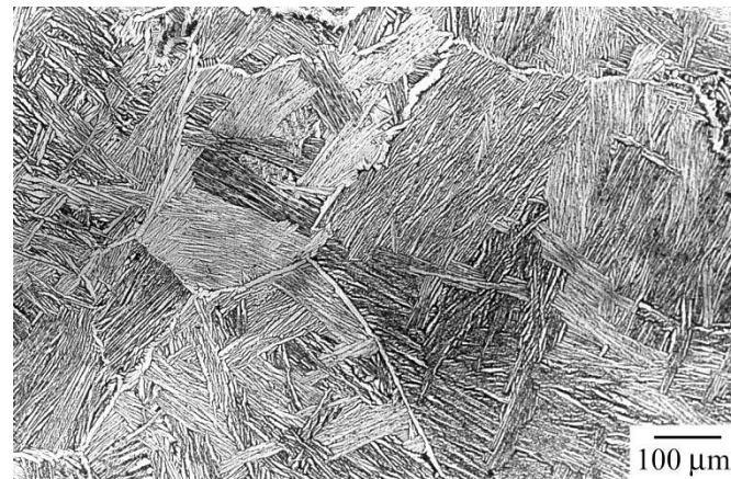
Optical micrograph of Ti-6Al-4V, \beta ht.-tr. at 1020°C/20min./FC showing Widmanstätten a structure with a phase present on prior \beta grain boundaries.
