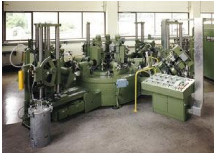
Figure 1.26 Example of 6 station rotary configuration
