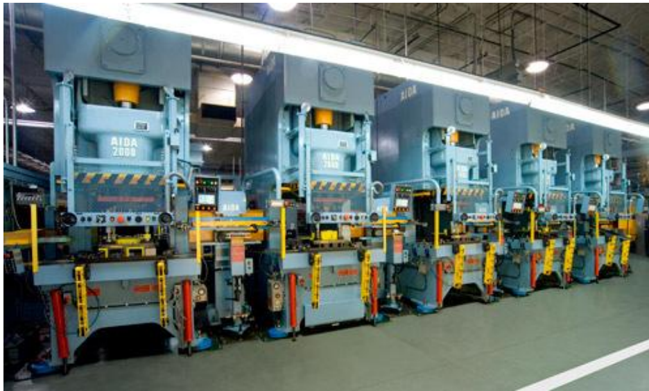
Figure 1.29 Example of 20 stations Transfer line
