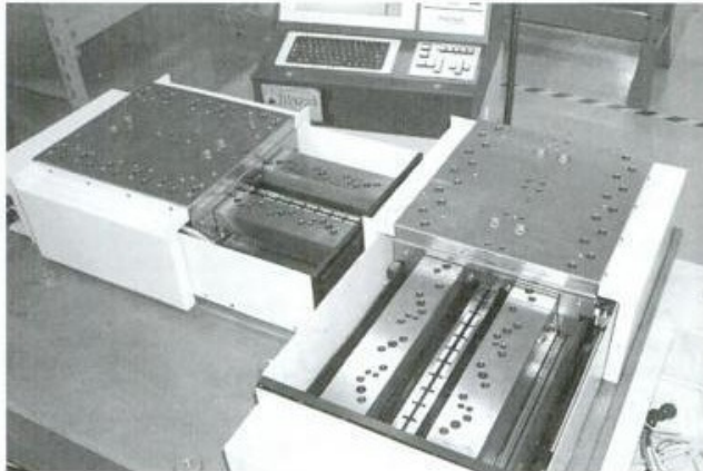
Fig. 5.23: A hydrostatic box type guideway for an ultra-precision machine [4].
