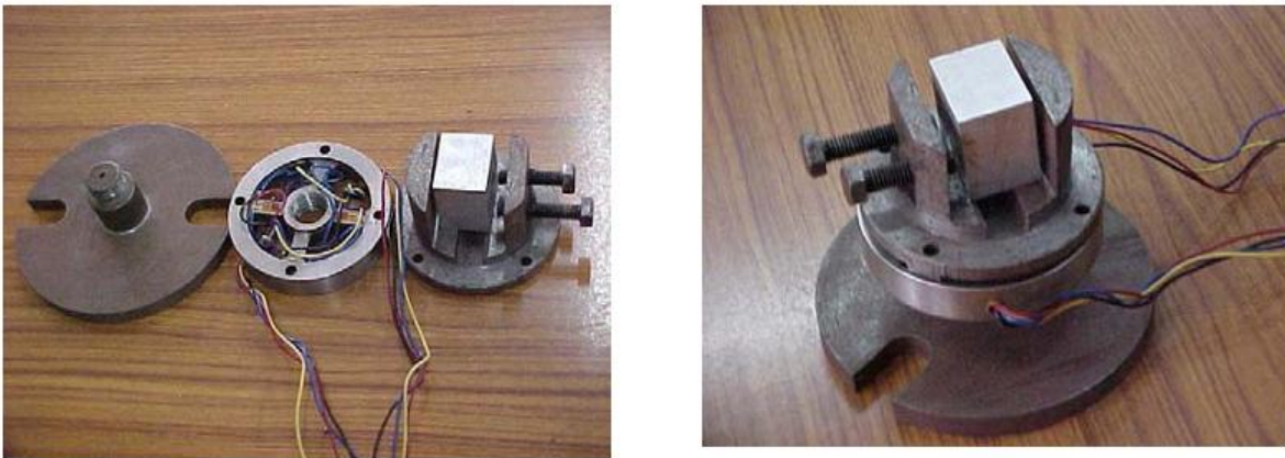
Fig. 2.19 A strain gauge type drilling dynamometer and its major components.
