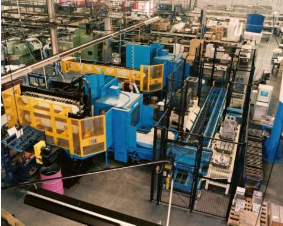
Fig. 68 A five-machine flexible manufacturing system for machining (photo courtesy of Cincinnati Milacron)
