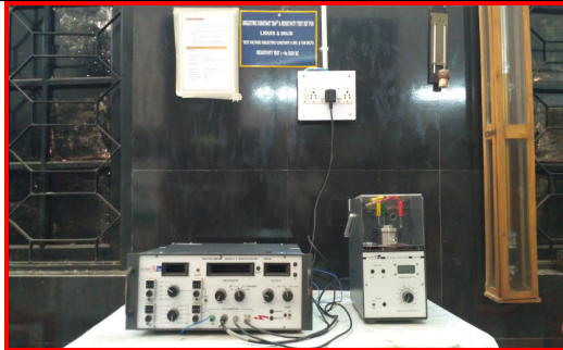
Dielectric loss factor ( \tan \delta ), capacitance and Resistivity Test Setup
